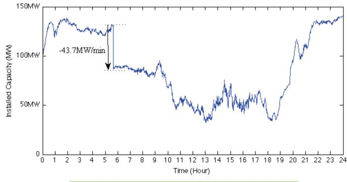
Wind output can drop 43.7 MW in 1 minute for a single 150-MW wind farm
