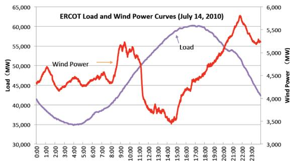
Fig. 2. The Load Profile and Wind Power Output of ERCOT [14]
