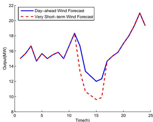
Fig. 3. The Wind Power Forecast Error in Near Real-time
