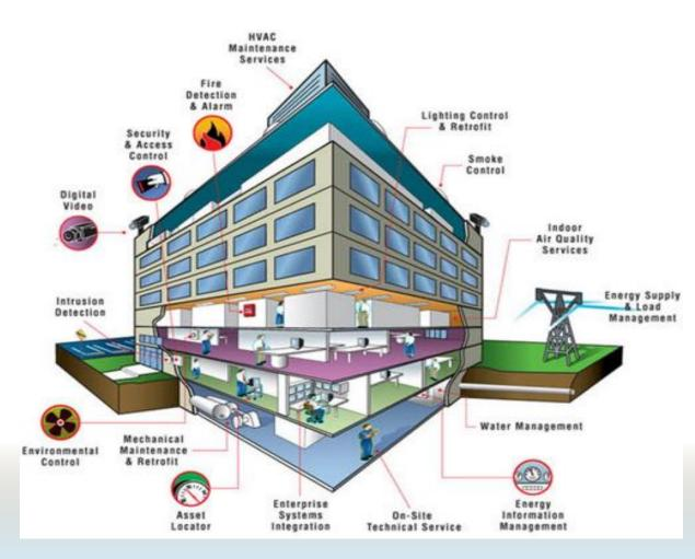
A single platform for monitoring and control of HVAC, lighting, water supply, sensor networks, security camera & fire emergency
